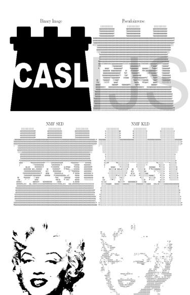
A test image (UCD CASL logo) and three ASCII art representations, which are created using the pseudo inverse and NMF utilizing the SED (Squared Euclidean Distance) and KLD (Kullback Leibler Divergence) cost function. Inspection of the logo text reveals that NMF preserves the curves best and minimizes black space. Furthermore, the selection of a different creates a different ASCII art representation
